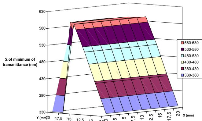
Figure 9. Mapping of the spectral shift of the wavelength of the minimum transmittance of G5TS37 obtained with the first set-up
