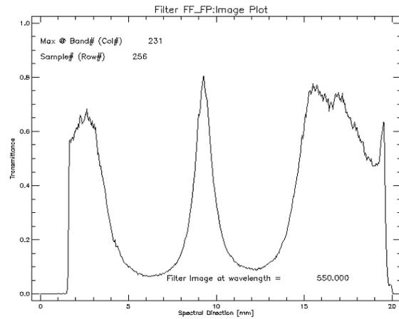
Figure 6.2 Transmittance profile along spectral direction at filter centre for the image at  $\lambda=550\text{nm}$
