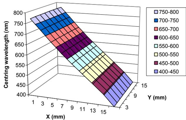
Figure 4. FF\_FP filter: Spectral shift of the transmitted peak through points 2mm-spaced points
