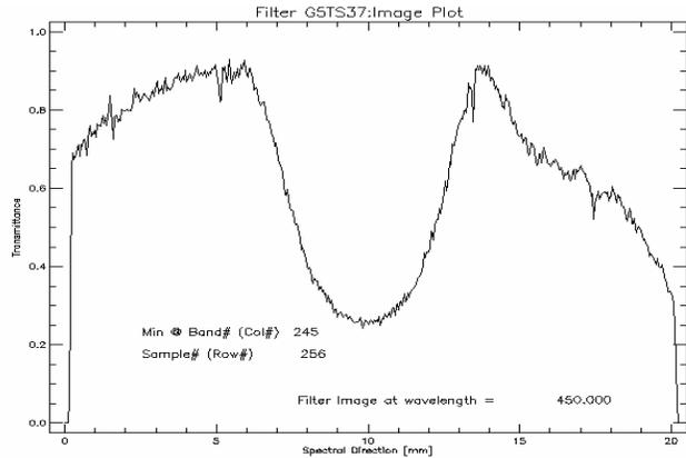
Figure 10.2 Transmittance profile along spectral direction at filter centre for the image at  $\lambda=450\text{nm}$
